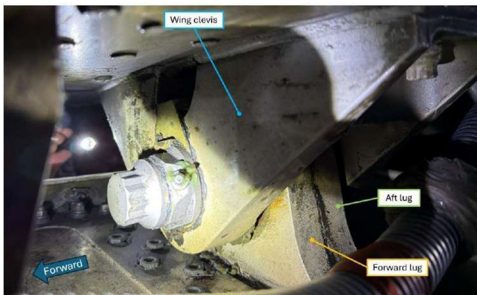
Figure 6. An exemplar installation of the pylon aft mount to the wing clevis. The aft mount spherical bearing is obscured by the wing clevis.
