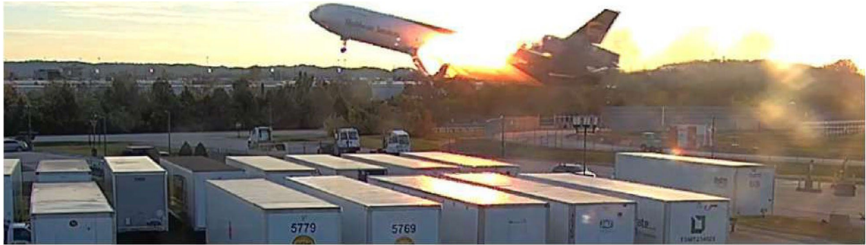
Figure 2. The fire in the area of the left pylon attachment to the wing continued as the airplane cleared the blast fence.
